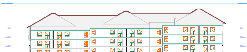
Attic space with different floor and roof levels
