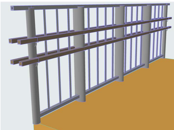
Two Handrails, Doubled
